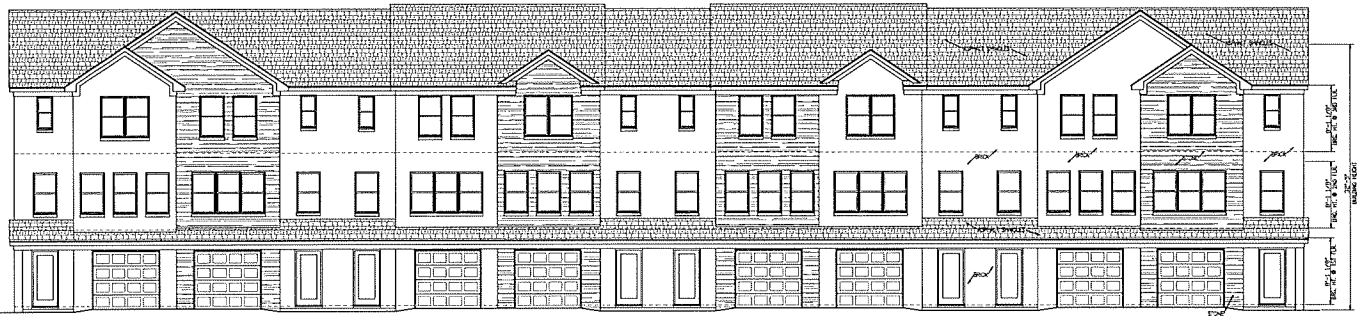
FRONT ELEVATION - 6 UNIT BUILDING SCALE: 3/16" = 1'-0"
