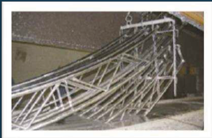
Superior Hot Dip Galvanizing Post Welding
