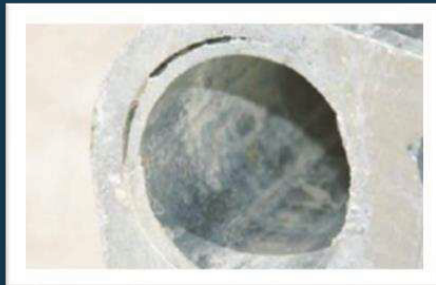
HDG After Fabrication Galvanized Inside and Out 100%
