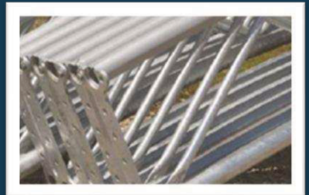
Completed Hot Dip Galvanized Trusses
